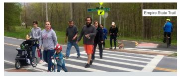
**Road Crossings—**a designated area where people walking and rolling can safely cross a roadway. To show where and when it is safe to cross, design options include roadway markings, crosswalks, curb extensions (aka "bumpouts") to shorten crossings, and visual indicators such as signs, flashing beacons, or traffic signals.
