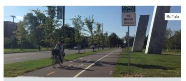
**Shared Use Path/Sidepath**—placed outside of a roadway surface and is physically separated from motorized vehicular traffic by a buffer or barrier. The path can be either within the roadway right-of-way or on an independent alignment. These are used by pedestrians, runners, micromobility users, skaters, wheelchairs users, and bicyclists.
