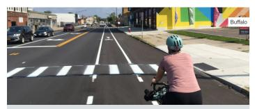
**Bike Lane—** a portion of a roadway designated for exclusive use by bicyclists using pavement markings and signs. Bike lanes are typically striped on both sides of a roadway and can either lie adjacent to the travel lane or separated from traffic by a striped buffer. They can be used on major roads to provide direct access to the same destinations that motorists seek.
